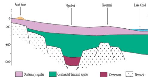
Fig. 2 Geological and hydrogeological formations in the lake Chad basin
