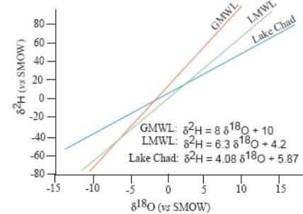
Fig. 4 Deuterium and oxygen-18 content compared to the global meteoric water line (GMWL)
