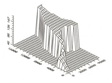
Figure 9. Modelling the water table elevation of the Gallikos aquifer (in metres).
