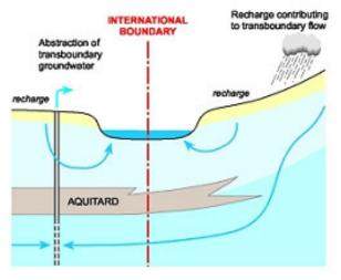
Figure 3. Interaction between transboundary surface and groundwater flows.
