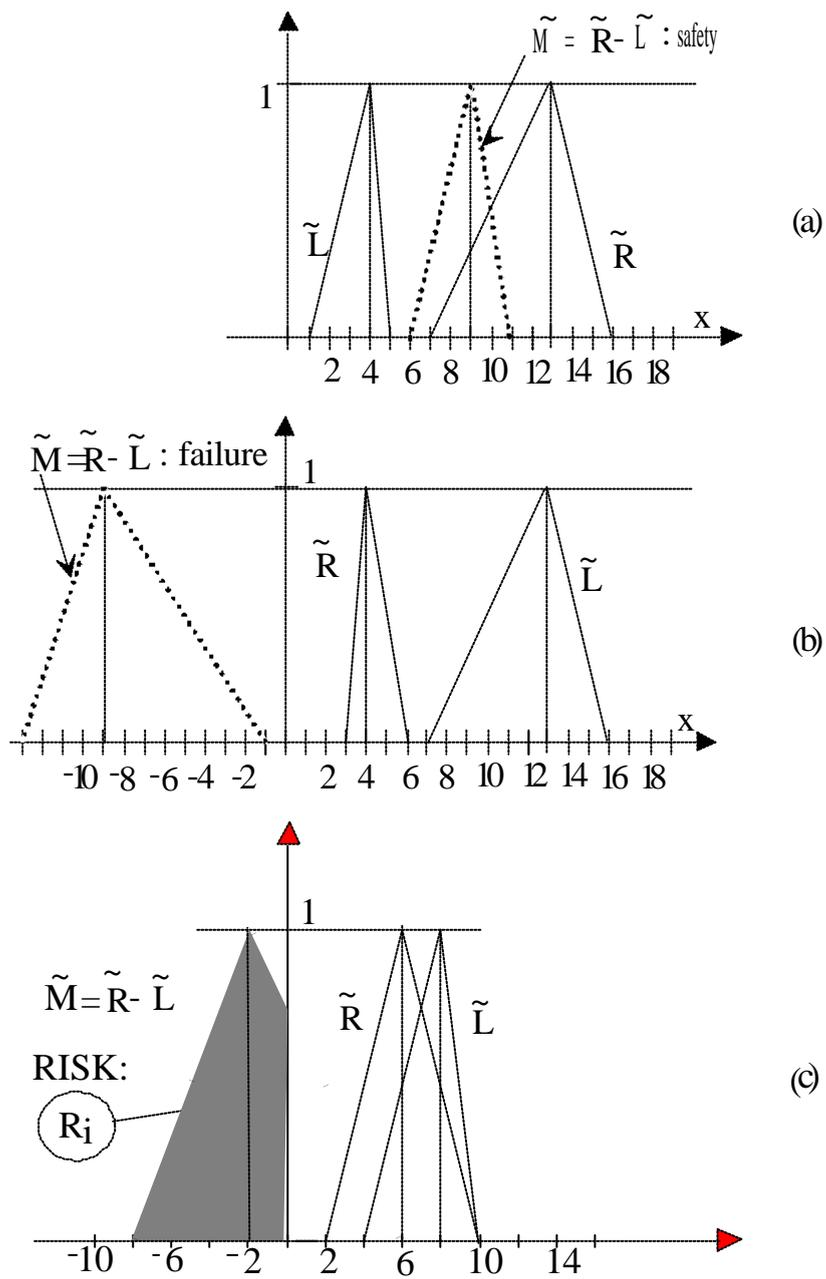
Figure 3. Absolute safety (a), absolute failure (b) and fuzzy risk (c).
