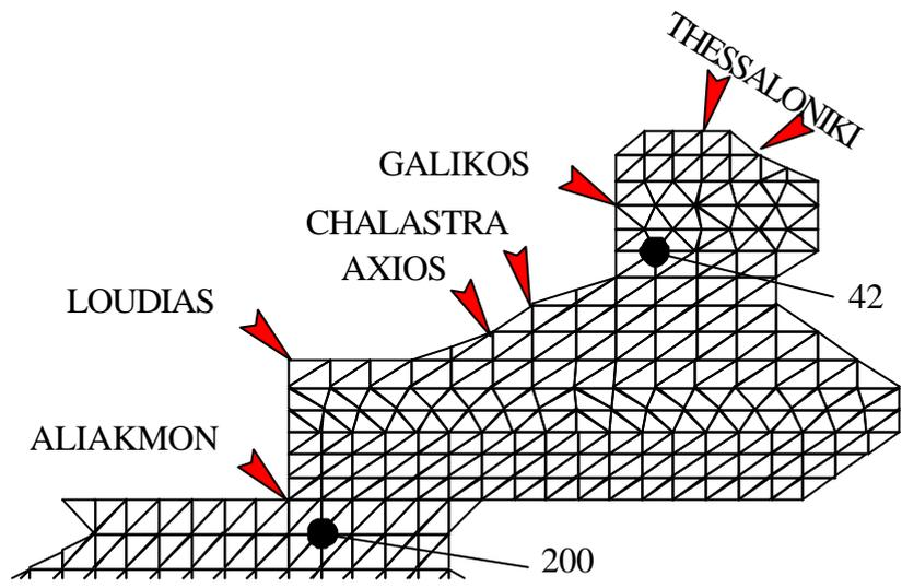
Figure 7. Finite element grid covering the Bay of Thermaikos
