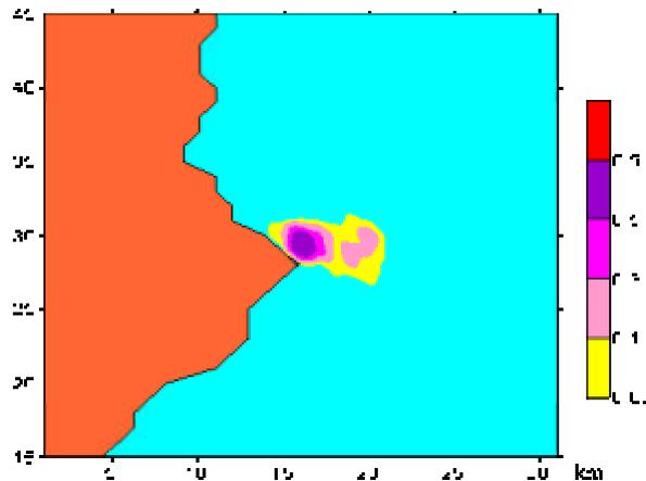
Figure 4. Contour lines of impact probabilities from a submarine outfall
