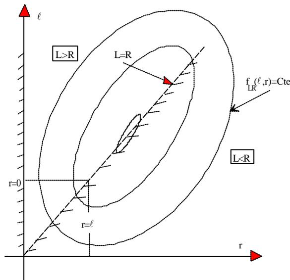
Figure 2. Calculation of the engineering risk by integrating the joint density probability function  $f_{LR}(\ell, r)$
